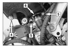
Remove the drain plug [4] on the oil tank and allow the oil to drain into a receptacle. Remove the screws [5] and tilt the oil return valve [6] to the side.
