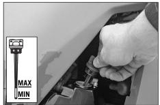
The oil level should fall between the lower end of the oil dipstick (MIN) and the MAX mark. The oil capacity between the MIN and MAX mark is 0.5 liters (0.13 USgal). Add more engine oil if necessary and check the engine for leakage.
