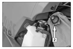
Carefully remove the radiator cap [2] with a rag, turning in a counterclockwise direction. The radiator should be completely filled with cooling liquid. No air should be in the radiator.
