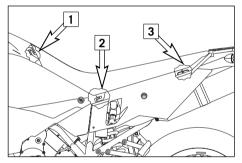
To remount, fit the nose [1] of the seat in the front, lower the back while pushing towards the front. Both noses [2] should fit into the frame. Insert the catch bolts [3] in the lock housing and push the seat down in the back until you hear the catch bolts snap into place. Check whether the seat is correctly mounted.
